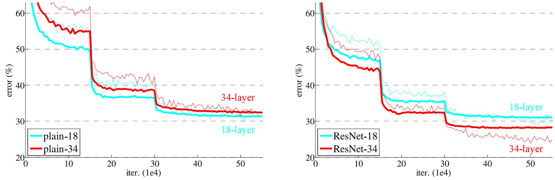
Figure 4. Training on **ImageNet**. Thin curves denote training error, and bold curves denote validation error of the center crops. Left: plain networks of 18 and 34 layers. Right: ResNets of 18 and 34 layers. In this plot, the residual networks have no extra parameter compared to their plain counterparts.
