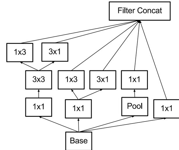
Figure 7. Inception modules with expanded the filter bank outputs. This architecture is used on the coarsest ( $8 \times 8$ ) grids to promote high dimensional representations, as suggested by principle 2 of Section 2. We are using this solution only on the coarsest grid, since that is the place where producing high dimensional sparse representation is the most critical as the ratio of local processing (by  $1 \times 1$  convolutions) is increased compared to the spatial aggregation.
