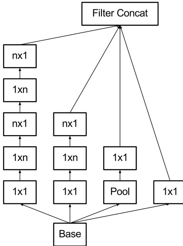
Figure 6. Inception modules after the factorization of the  $n \times n$  convolutions. In our proposed architecture, we chose  $n = 7$  for the  $17 \times 17$  grid. (The filter sizes are picked using principle 3)
