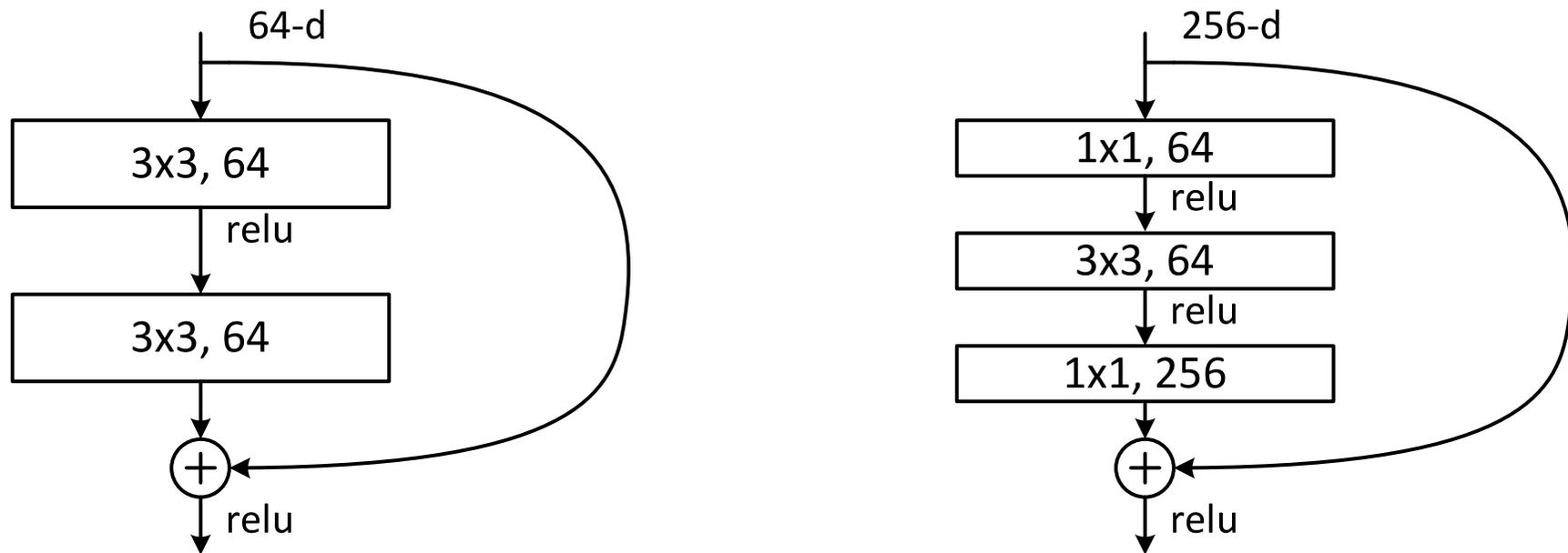
Figure 5. A deeper residual function  $\mathcal{F}$  for ImageNet. Left: a building block (on  $56 \times 56$  feature maps) as in Fig. 3 for ResNet-34. Right: a “bottleneck” building block for ResNet-50/101/152.
