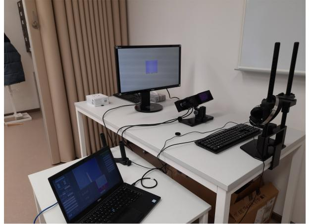
Figure 4: EMMT: Experiment setup with eyetracker (EEG and audio recorder not shown).
