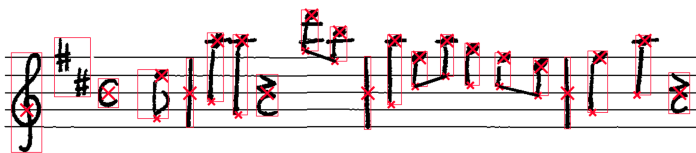
Fig. 8. Groups with bounding boxes. Large crosses mark symbol origins, smaller crosses mark where a stem ends and a beam attaches. A key signature has no anchor point.
