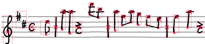
Fig. 5. Canvas Items (the red boxes) form the basis of horizontal spacing. The red crosses denote key positioning points, such as notehead centers and stem tops.
