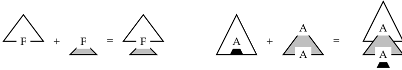
Figure 3.5: Tree substitution at a frontier node F and tree adjunction at an internal node A.
