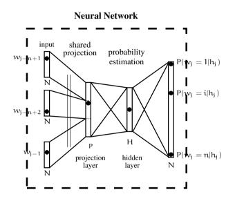
Figure 1. Architecture of the continuous space LM.  $h_j$  denotes the context  $w_{j-n+1}, \ldots, w_{j-1}$ . P is the size of one projection and H,N is the size of the hidden and output layer respectively. When short-lists are used the size of the output layer is much smaller then the size of the vocabulary.
