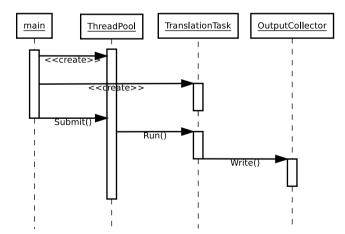
Figure 1. UML Sequence diagram for multi-threaded Moses mainline
