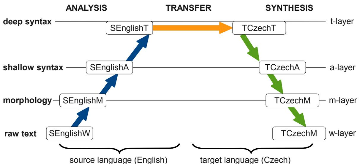
**Figure 2.** Vauquois diagram for translation with transfer on the tectogrammatical layer
